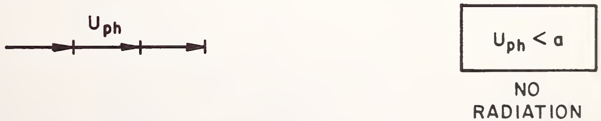
FIG. A-2. EFFECT OF RATIO OF PHASE SPEED U_{ph} AND SOUND SPEED a ON RADIATION
